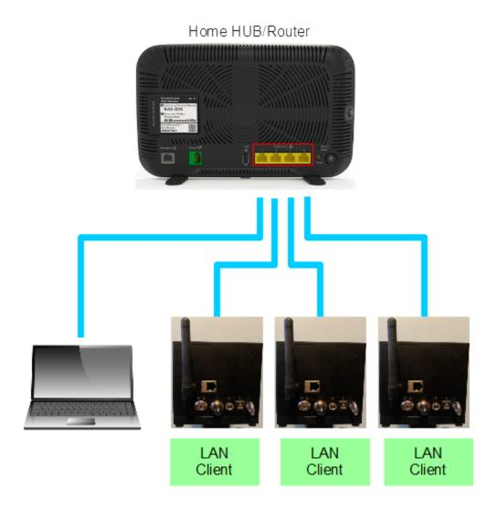
This configuration could also be used with an additional network switch in order to increase the number of available ethernet ports, allowing more network laser cubes to be connected.
